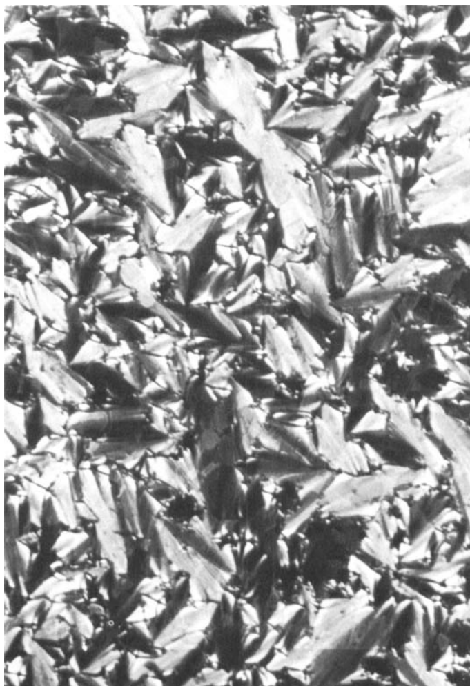
Figure 5. PdC76ET, smectic A phase at 477 K, crossed polarizers.
