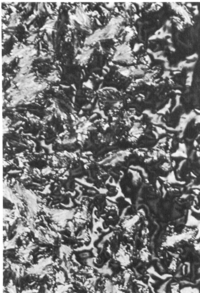
Figure 4. PdC76ET, smectic C phase at 460 K, crossed polarizers.
