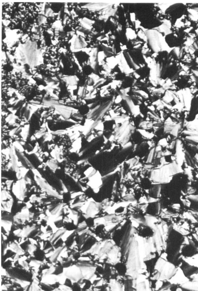
Figure 3. CuC9ES, smectic phase at 463 K, crossed polarizers.
